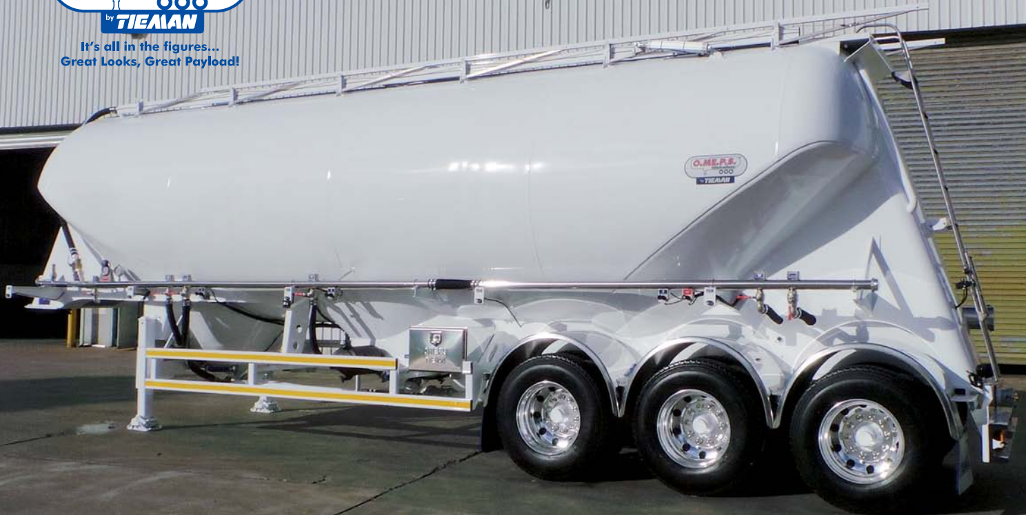
42CM aluminium cement tanker
