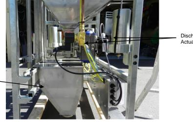
Discharge Valves and Actuators
