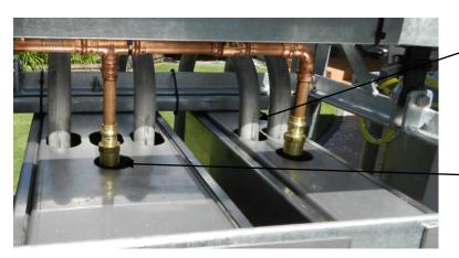
Admixture feed pipes – no contact with weighing mechanism
